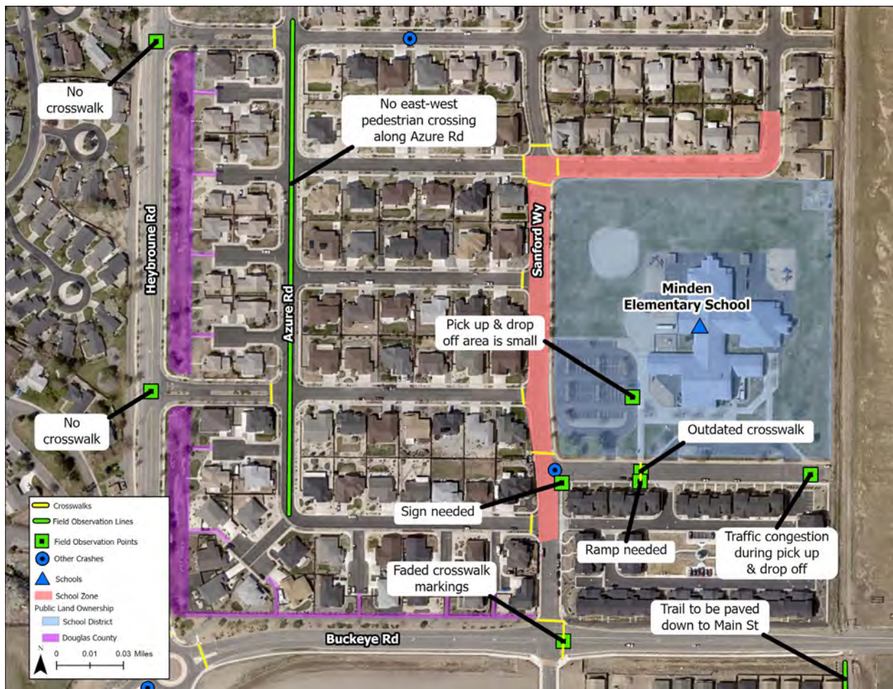
Exhibit F-1: Minden Elementary School Existing Conditions
